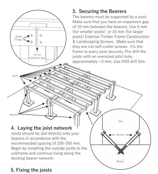
Fix the joist into the bearers. Use a 6–10 mm single thread External Timber screw to ensure proper fixing and pre-drill the material with an oversized pilot hole, approximately 3 mm. Use HSS Drill bits. As an additional support, you can fix noggins between the joists. When joining two joists, ensure an expansion gap of 10 mm is left. Where two boards are expected to meet, ensure sufficient support is provided in the form of a double joist.
